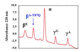
β<sup>A-T87Q</sup>-globin allows for monitoring of protein levels produced using HPLC
